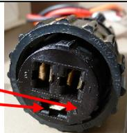
This depiction is the female connector to attach to the Boss "R" wiring harness.
